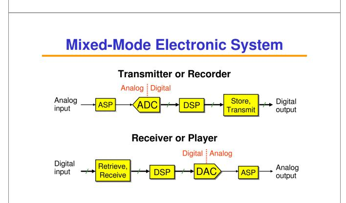
• Usually, the ADC, DAC and ASP blocks limit the accuracy and bandwidth.
