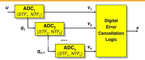
• Purpose of error cancellation logic is to eliminate quantization noise from all stages, except the last, so that:
